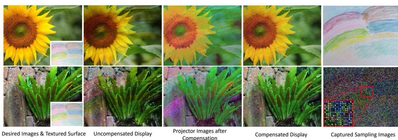
Figure 1: Projection display results of two images ('sunflower' and 'plant') on a color textured surface using our radiometric compensation method that requires capture of only two images to generate a more accurate compensated image as opposed to capturing tens or hundreds of images required for any existing method. From left to right: The two desired original images and the color textured surface (1st column); the display results without radiometric compensation (2nd column); Our input projector images computed using our radiometric compensation method (3rd column); The projections display results with our radiometric compensation (4th column); the two images used in our radiometric compensation method (5th column).
