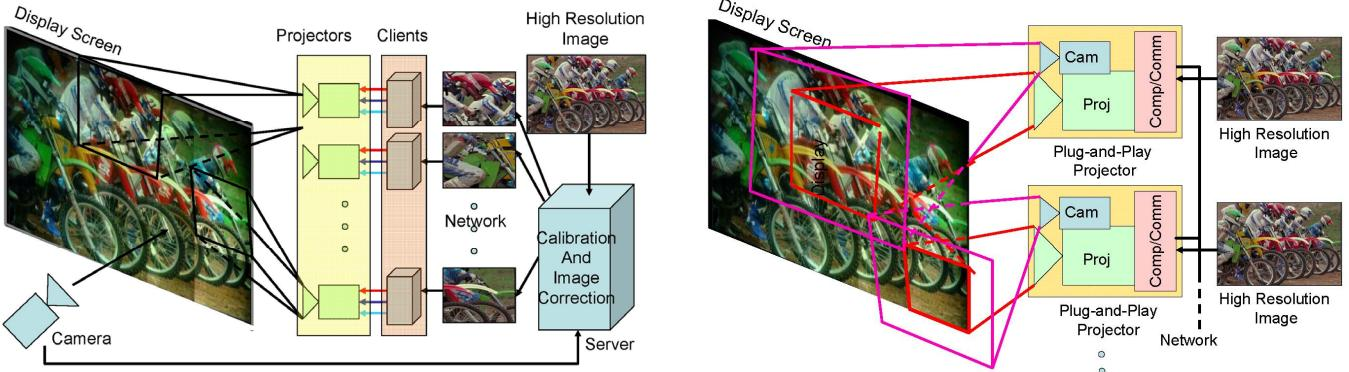
**Figure 2.** A centralized architecture for multi-projector displays (left) and a decentralized architecture using plug-and-play projectors (right).
